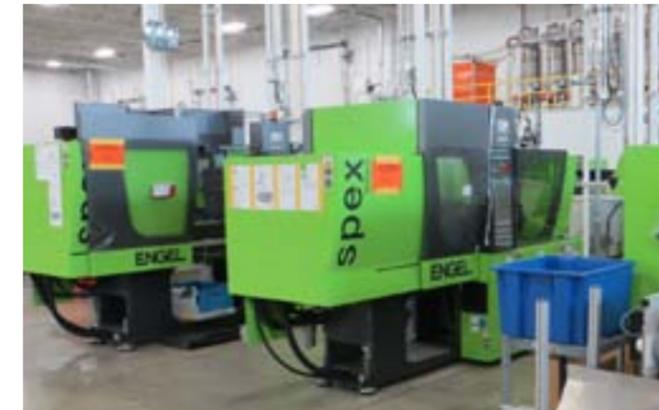
Asyst Technologies has purchased two 85-ton clamping-force and two 55-ton clamping-force injection molding machines since March 2013. The machines were made and shipped to the U.S. by Austrian company Engel.
